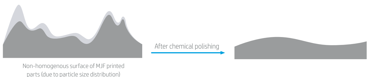
Figure 15. Surface roughness improvement after chemical polishing
