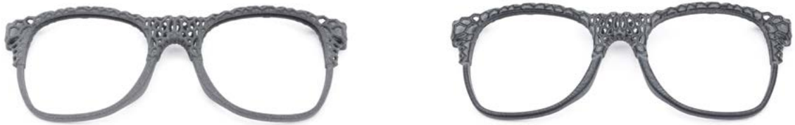
Figure 11. HP Multi Jet Fusion part before (left) and after tumbling (right)
