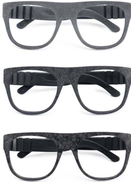
Figure 16. Image of raw part, and two chemically polished parts with varying degrees of processing
